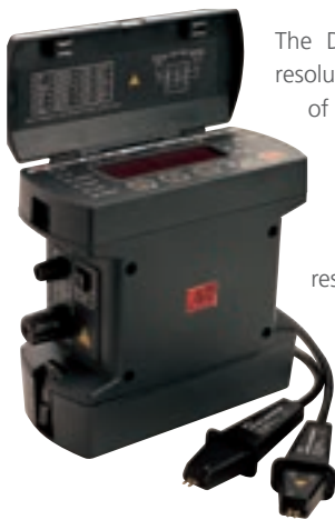
DLRO10 has bright 4½ digit LED display making it easy to read under all lighting conditions
